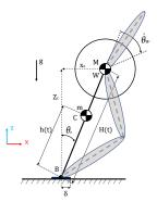
Fig. 1. Linear Inverted Pendulum Plus Flywheel Model.
